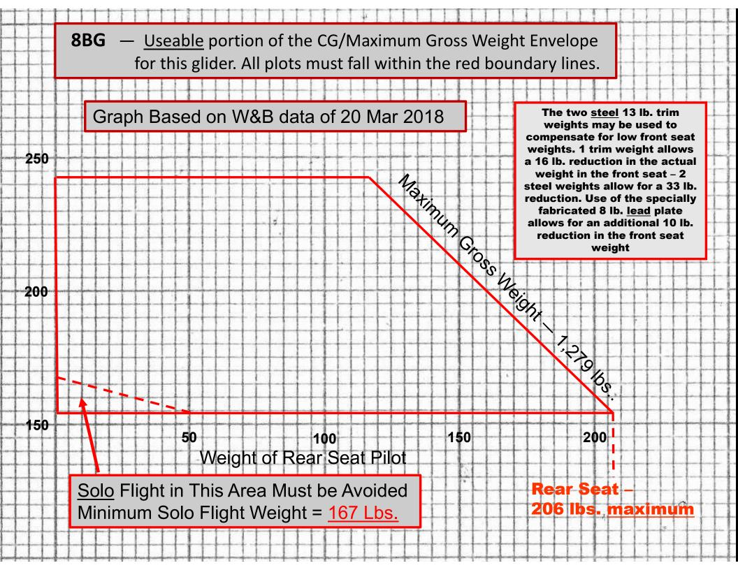
Specific to 8BG - Because the trim weights are installed at a location that is somewhat forward of the front seat, both their <u>actual weights</u> as well as their <u>weight change effects</u> must sometimes be taken <u>separately</u> into account. Neither does the Flight Manual identify the station where these weights may be installed. (Computations and measurement reveal this station to be approximately 59 inches forward of the datum.)
