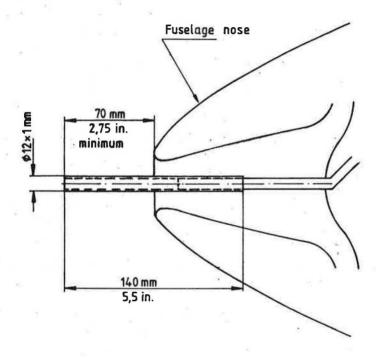
Brass tube 5,5 in = 140 mm in length (12  $\emptyset$  x 1). One may also use a suitable plastic tube provided that it is sufficiently stiff and straight.
