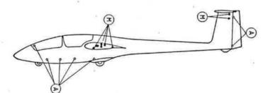
OIL: machine oil or car engine oil LUBRICANTS: multi purpose grease
