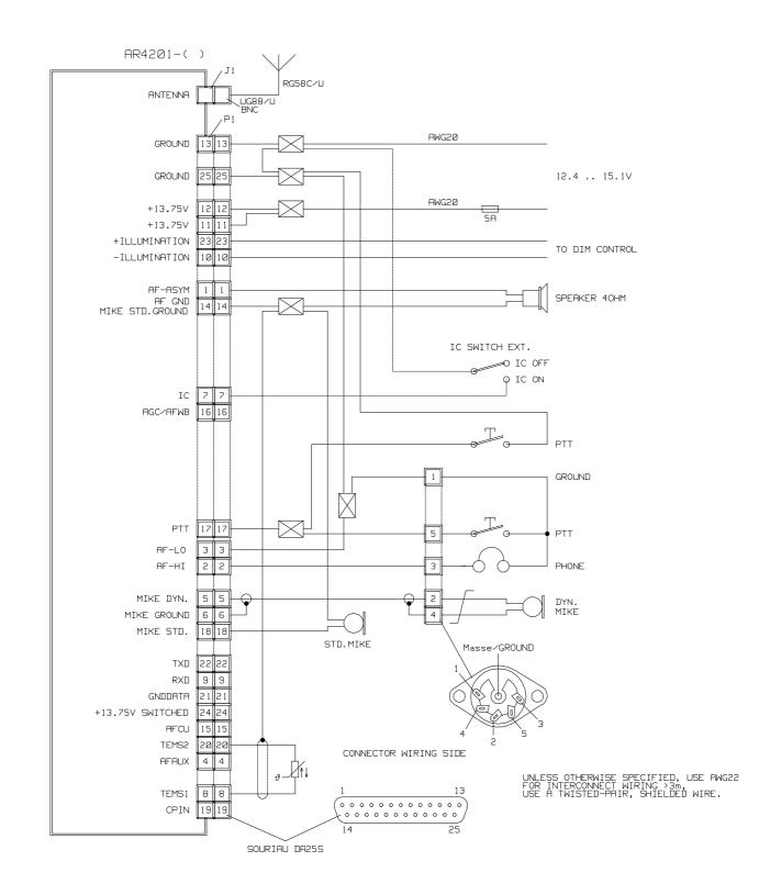
Fig. 2-4 Interwiring of the VHF transceiver with dynamic mike
