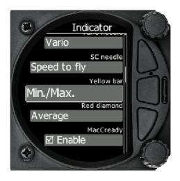
Vario Needle: Can be set to Relative, Netto, Speed to Fly or Vario SC needle: Can be set to Relative, Netto, Speed to Fly or Vario Yellow Bar: Can be set to G-meter, Min/Max vario or no bar
