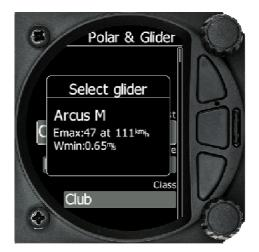
You can modify the polar by changing coefficients **a**, **b** and **c**. A polar is defined as a quadratic equation with the parameters a, b, and c. Use the SeeYou program (Tools->Polar) to calculate coefficients a, b and c for a given glider's polar. The program requires three sink points entered at selected speeds (e.g.: 100 km/h, 130 km/h, and 150 km/h). The program will calculate the values of a, b and c, which should be noted and entered into the LXNAV S80.
