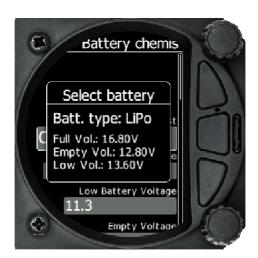
Alternatively you can manually change the Full Voltage, Low Battery Voltage and Empty Voltage if your battery type is not listed.
