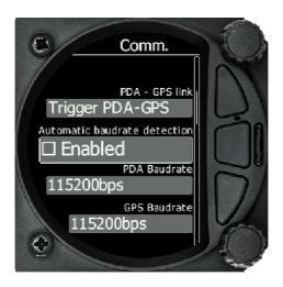
Each port can be configured separately. If your PDA device does not support automatic switch to DIRECT LINK between GPS and PDA port, here is manual **GPS-PDA link** menu. When **autobaudrate** is enabled, the LXNAV S80 will automatically search on all speeds to receive valid data. When the S80 receives a valid NMEA sentence it will lock on that baudrate and stop searching. In case that communication is lost LXNAV S80 will start again searching on all baudrates.
