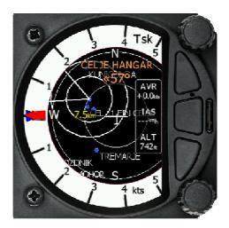
You can also change the Observation zone from the defaults for each Waypoint. To do this, select the waypoint in the task and then press the bottom rotary knob. The quick access menu allows you to insert, edit, delete or change the zone for the Waypoint. If you select **Zone**, you can modify the zone for that specific waypoint only.
