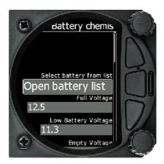
Batteries used in gliders today are not just the old style lead acid battery but also Lithium IIon (LiIon) and Lithium Iron Phosphate (LiFePo). Each battery type has a different power delivery curve and it is now possible to configure the Low and High Battery warnings
