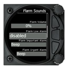
Flarm Volume: can be adjusted with the slider
