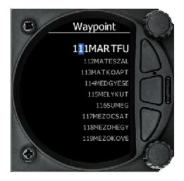
The Waypoint can be selected from the alphabetical list of waypoints. (See uploading files section 5.6.14.1). Rotating the bottom rotary knob moves you through the
