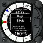
Rotate the bottom knob to modify any setting. Next, check the safety altitude (height above destination, arrival altitude) setting.
