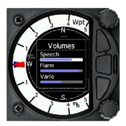
The lower rotary knob is used to adjust settings, within the current screen display or within menus. With the lower rotary pushbutton, we can toggle between MC, Bal and Bugs settings. In all other menus, this knob is used for setting values and editing texts.
