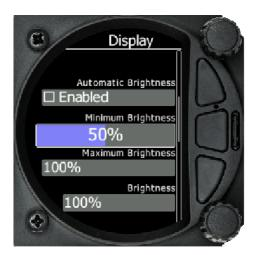
With a push of the rotary button you can activate the slide control, then with rotation of the knob you can select the preferred value and confirm it with the push button.
