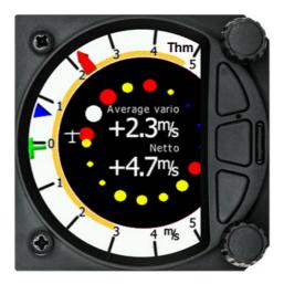
The Thermaling Assistant displays a graphical representation of your location within the thermal, Large red bubbles indicate the strongest part of the thermal and small blue dots indicate the weakest part of the thermal. The point of strongest lift is indicated by a white large bubble. The Thermaling assistant can be set to automatically change to the Thermaling assistant page or be manually selected.
