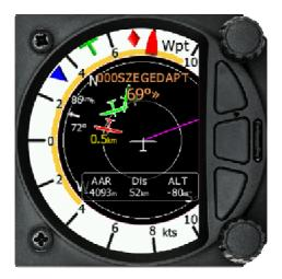
The first page shows a line to a selected waypoint, the name of the selected waypoint at the top of the screen and the relative bearing and chevrons indicating the direction to turn towards the selected waypoint. (The Navboxes can be configured with distance and arrival Altitude.)
