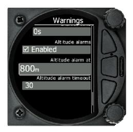
The warnings dismiss time can be set from 0 to 120 seconds
