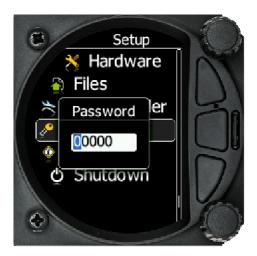
Turn the bottom rotary Knob to set the character and then press the enter key (bottom key) to move to the next character to the right. Press the escape key to move back to the left. When you have finished editing, press the Enter key. Short-press the bottom rotary knob to enter or exit an edit field ("control").
