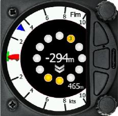
The central number and chevrons indicate if the Flarm target is below or above and by how many meters/feet. The number in the bottom left indicates the range in meters/feet.
