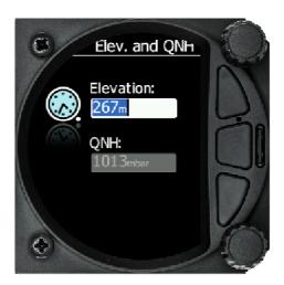
The instrument will offer elevation over standard pressure level QNE. Use the knob to finetune the elevation.
