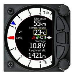
The navigation boxes in this second task page can be changed using the quick access menu and selecting **Navbox**. You can make changes to the Navboxes as described in chapter **5.3.2.**
