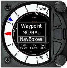
To **Select** a waypoint, rotate the bottom rotary knob to highlight the select option and then press once. This will open the Waypoint list
