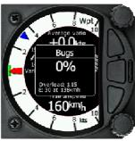
To change the MacCready value, rotate the bottom rotary knob. A short press on the bottom rotary knob moves to the Ballast box and stores the MacCready setting. Pressing the bottom rotary knob again will open the Bugs box. If no action is performed for 3 seconds, the box will close.
