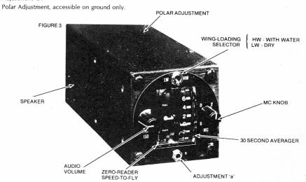
If the pilot wishes to thermal, or just fly around, he should follow the variometer only, which can be left in any sensitivity desired, and ignore the Speed-to-fly Zeroreader. Or he can follow the Audio.
