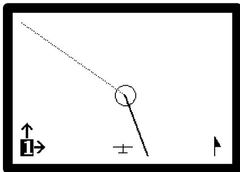
This illustration shows the turnpoint cylinder you would see approaching a turnpoint from the south, with the moving map displaying Nose-Up. The heavy line is your current task leg, and the dotted line is the next leg. The glider is left of the course line.
