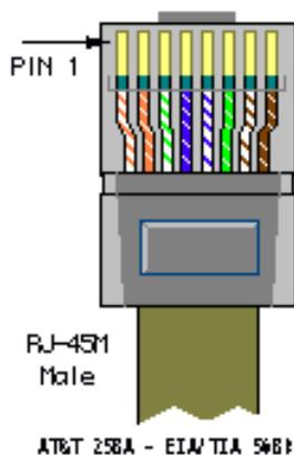
If you have a cable with standard computer network color coding, the colors will match this diagram and the table below. If not, carefully use the pin numbers to determine the correct connections.
