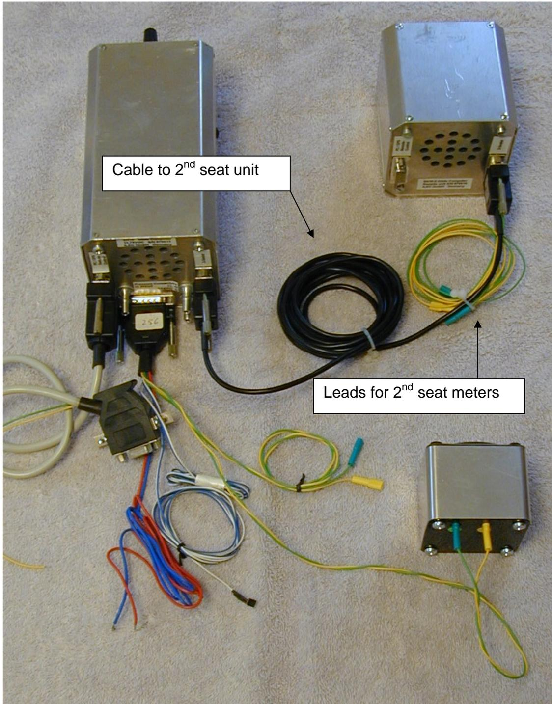
The SN10 has three electrical connectors at the rear of the instrument. Their connections, and also the color codes for the ILEC-supplied cables follows.
