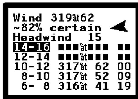
The illustration shows the wind measurement during a wave flight in very strong winds. The wind is currently from 319 degrees true at 62 knots. The wind is now almost off the right wingtip, so the instantaneous headwind is just 15 knots. The average in the 10,000 to 12,000 foot altitude band is from 317 degrees true at 62 knots, and the data for this altitude band was last updated 00 minutes ago. The information about the 8,000 to 10,000 foot altitude band is now 09 minutes old.
