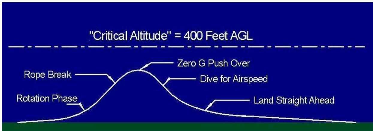
The words "*as far below the horizon as above it*" have been carefully chosen to work, so the maneuver will work in all cases. They mean exactly what they say. If a rope break occurs at 20 feet with the nose up 10 degrees, the glider will strike the runway if the pilot attempts a 45 degree nose down recovery. At 500 feet, with the nose up 45 degrees above the horizon, lowering the nose only 10 degrees will not result in a safe recovery.
