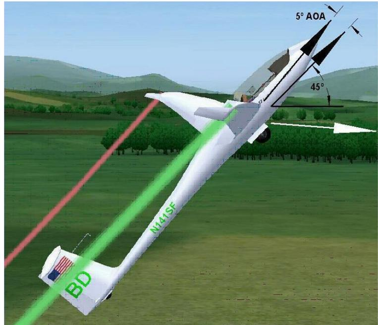
If it is seen that a wing tip will touch the ground despite corrective aileron input, the pilot should release and not try to "save" the launch. Failure to do so may result in a particularly ugly ground loop which may end with the glider crashing inverted. The CG release does not help keep the glider rolling straight as does a nose hook.
