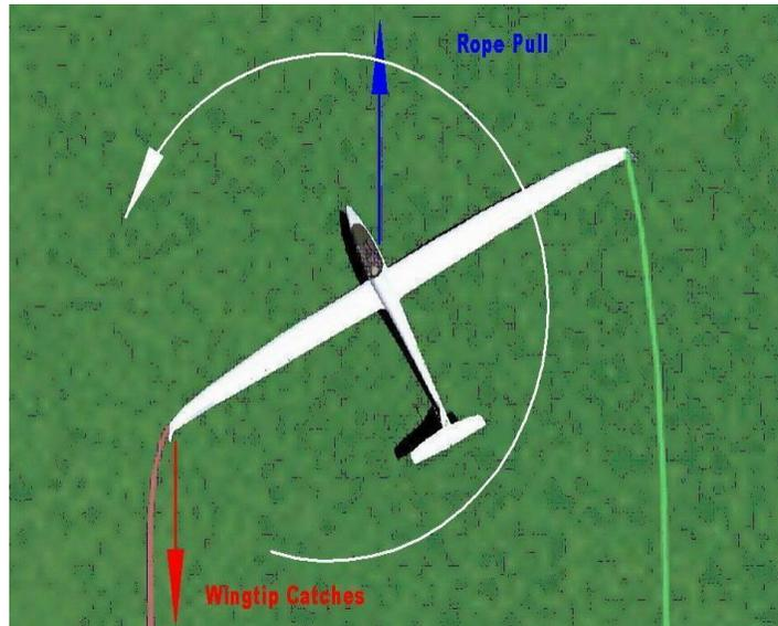
The vast majority of winch launch accidents occur due to wing drop during the takeoff roll or a stall spin after a launch failure. Do not continue the launch if **anything** abnormal occurs. Above all else, when a launch failure occurs, FLY THE GLIDER!
