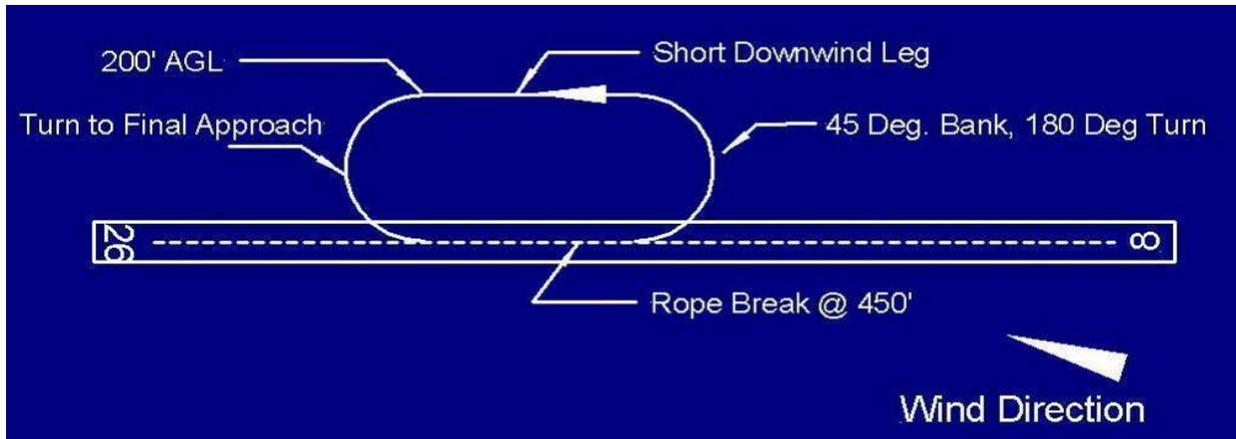
With most runways, there is an overlap where either a straight ahead landing or a circle is possible. A straight ahead landing is always preferred for safety reasons. When landing straight ahead, the pilot should make an attempt not to land on the rope.
